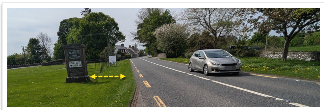
Figure 2.2 – Davitt Museum Sign May Prevent Barrier from Deforming Following Vehicle Impact
